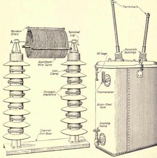
Fig. 182.—Air-insulated choke coil for pressures up to 150,000 volts.
